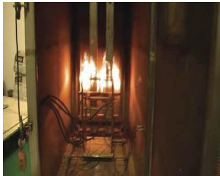
Clause 8.2.14 : Verification Resistance to Flame Propagation
