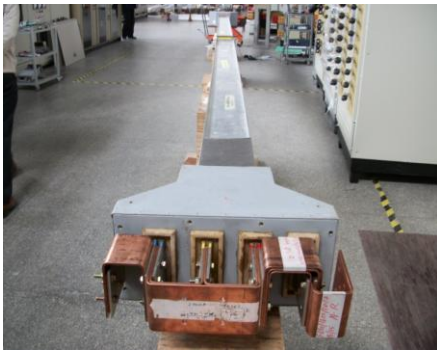
Clause 8.2.13 : Verification of Electrical Characteristics of Busbar Trunking System
