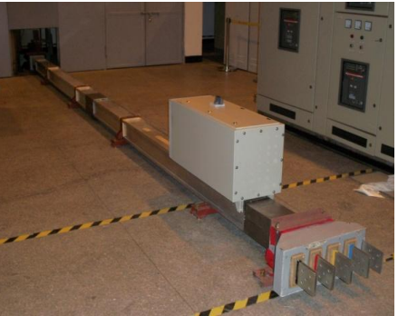
Clause 8.2.3.2.3a : Verification of Short Circuit Strength (Icc) - Feeder Elements without Tap-off Unit
