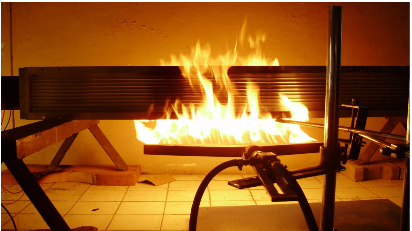
IEC 60331-3 : Test for Electric Cables under Fire Condition-Circuit Integrity (with Conductors Energised)
