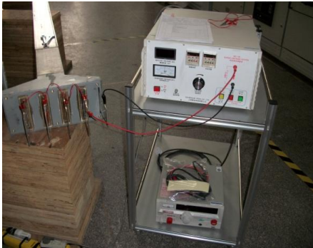
Clause 8.2.2 : Verification of Dielectric Properties
