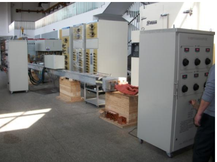
Clause 8.2.6 : Verification of Mechanical Operation
